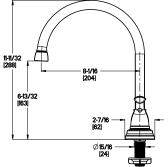
Ø1-3/8 Min to Ø1-1/2 Max. Deck Hole Openings
